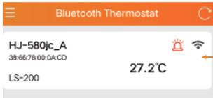
Click here to connect to the product. On this page, if you short press the defrost button on the controller, a red background will display a prompt. This function is used to identify the device when multiple devices are not connected
